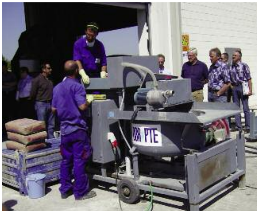
Spanish BBR Network member BBR PTE's grouting plant.
