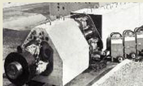
ABOVE: Construction of bottom cap with buttresses for anchorages of the UK's Dungeness B pressure vessel. BELOW: Testing of BBR anchor head. Stressing device consists of three 500t jacks, hydraulic pumps and load cells.
